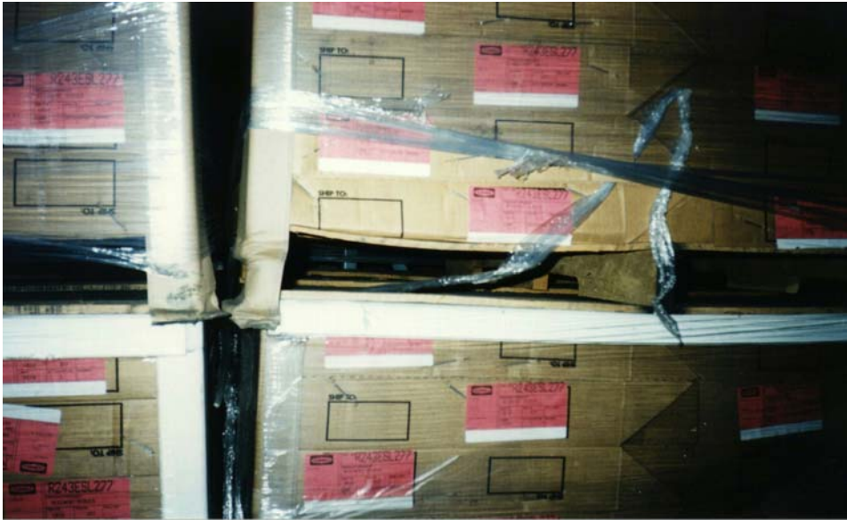
Figure 4: Top Deck bending between the stringers of this lightweight pallet design creates stress concentrations on the packaged product
