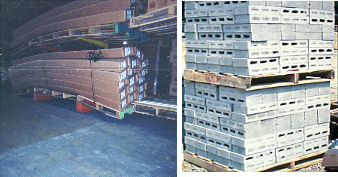
Figure 5: Examples of products with low load bridging and high load bridging characteristics
