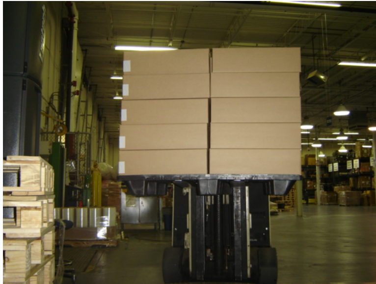
Figure 6: Column stacked boxes remain stable on the low stiffness plastic pallet during handling due to a tie sheet between the 3 rd and 4 th box layers.
