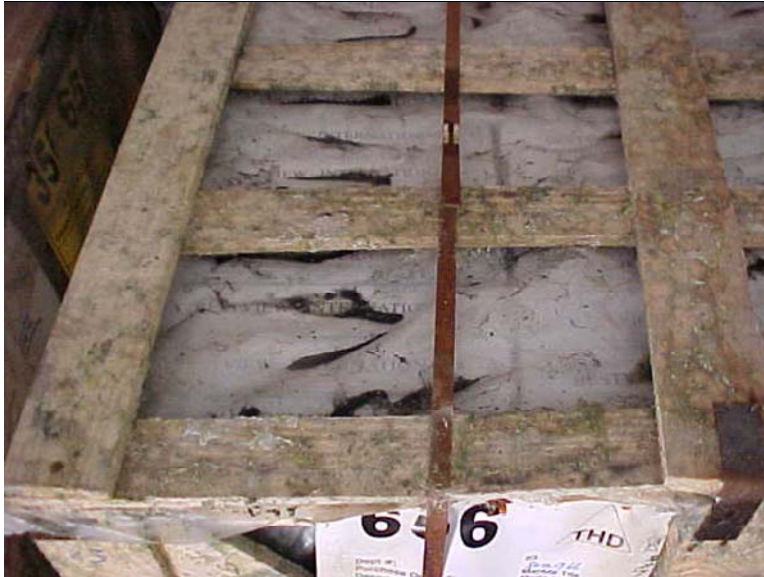
Figure 3: Green mold, white mold, standing water, and banding corrosion from excess moisture after overseas shipment inside an ocean container.
